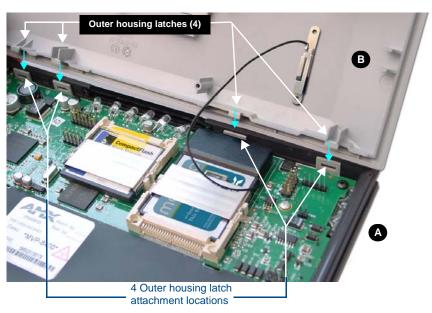
FIG. 12 Outer housing latch attachment locations
